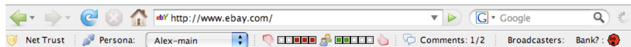
Figure 1: The Net Trust toolbar displays aggregate negative evaluations (red lights on left), aggregate positive evaluations (green lights on right), a comment count, a ratings count, and third-party (broadcaster) evaluations. A full ratings window with friend evaluations is available on demand.
